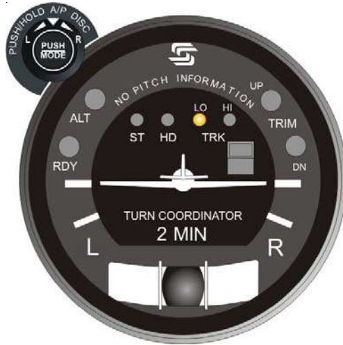
Fig. 2-23. AP Display, LO TRK Mode Engaged (System Thirty)
