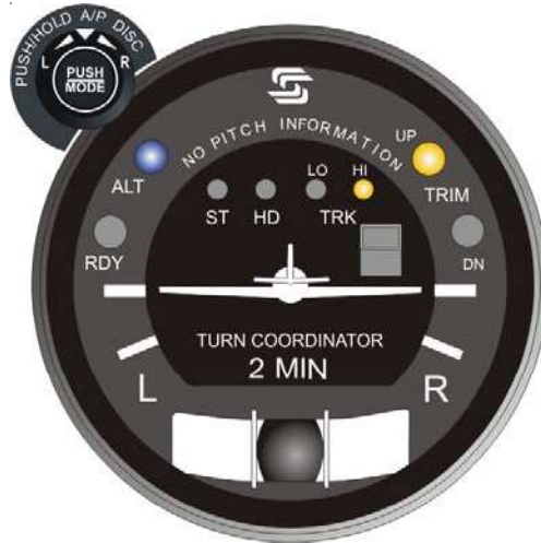
Fig. 2-26. AP Display, HI TRK and ALT HOLD Modes Engaged, TRIM UP Required (System Thirty)
