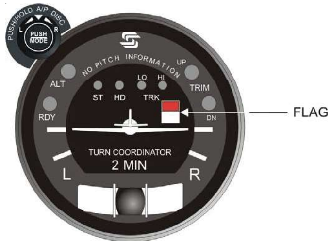
Fig. 2-12. AP Display, Low Voltage Flag (System Thirty)
