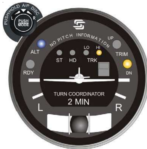
Fig. 2-27. AP Display, HI TRK and ALT HOLD Modes Engaged, TRIM DN Required (System Thirty)
