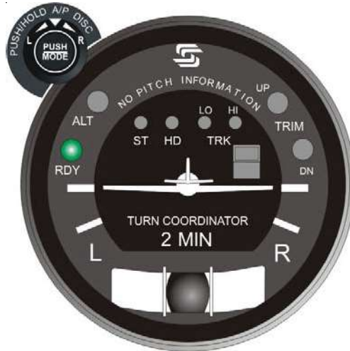
Fig. 2-10. AP Display, RDY for Operation (System Thirty)
