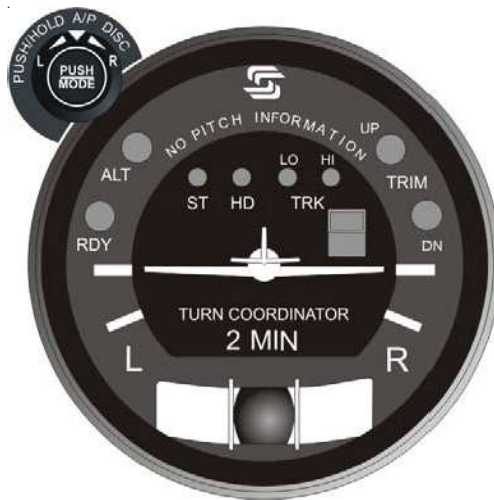
Fig. 2-11. AP Display, Turn Coordinator Failure (System Thirty)
