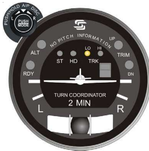
Fig. 3-3. AP Display, LO TRK Mode Engaged
